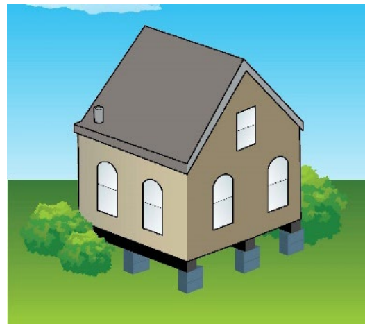
Figure 2. Schematic of a block and beam foundation.
